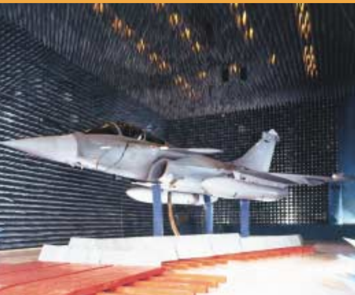
Rafale measurements in anechoic chamber.
