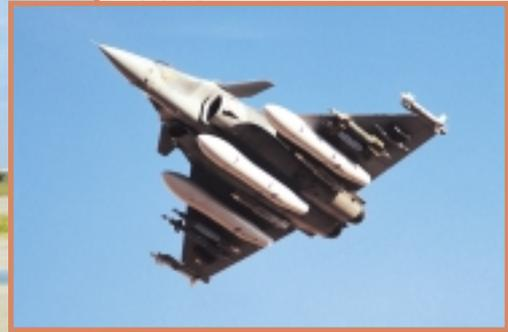
**GBU-12s - included here in a swing-role configuration - provide precision strike capability with minimal collateral damages.**
