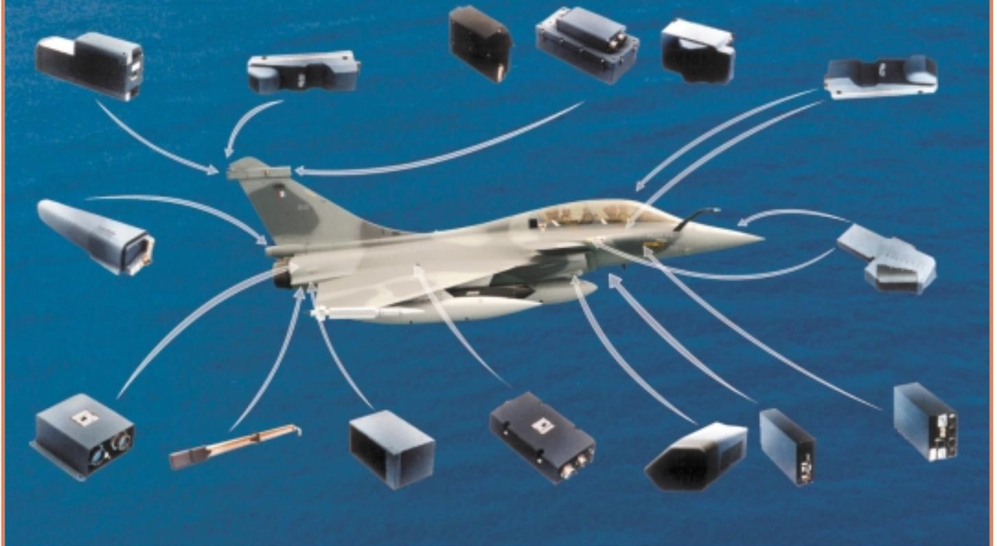
*The Spectra System and its various components, on board the Rafale.*
